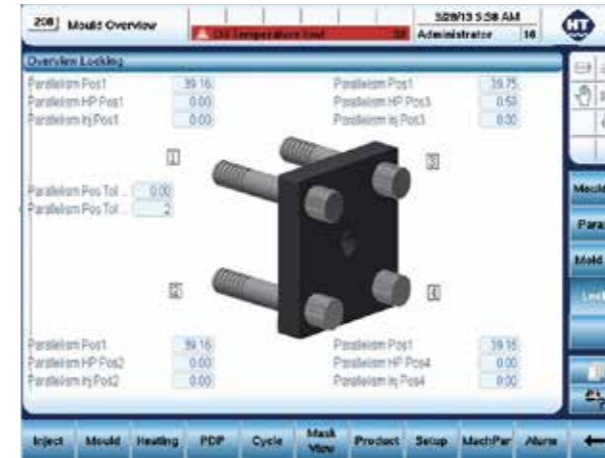
Platen parallelism monitoring for effective protection of the mold and smooth operation of the machine
