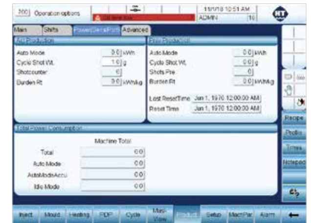
Energy control and monitoring over the production process and equipment operation status
