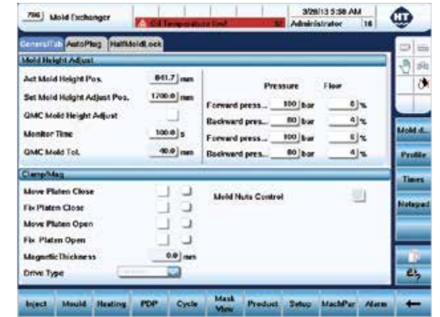
Integrated one-key mold exchange control for unmanned process exchange and improved productivity
